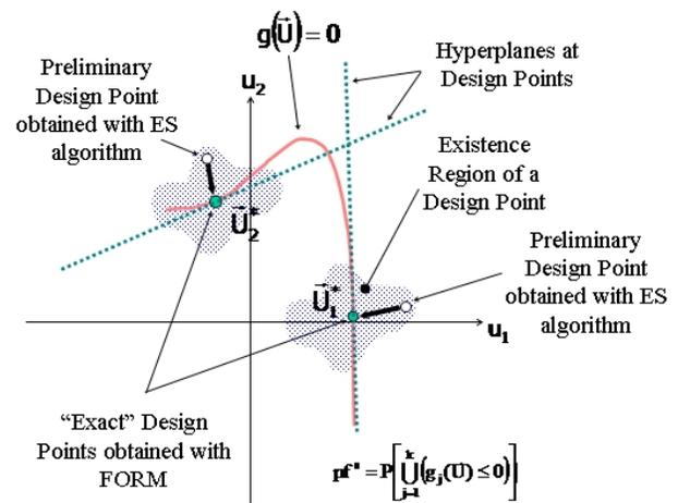
Figure 2. Schematic representation of the proposed methodology
