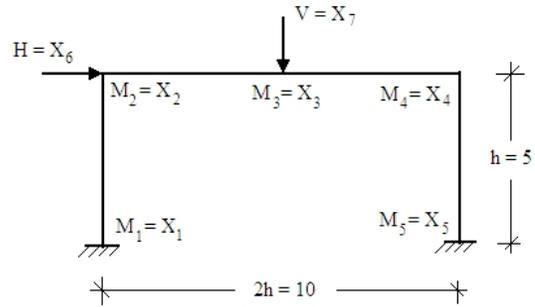
Figure 8. Plane frame structure ( $M_i$ , node bending strength)
