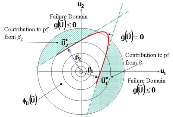
Figure 1. Limit state function with two design points
