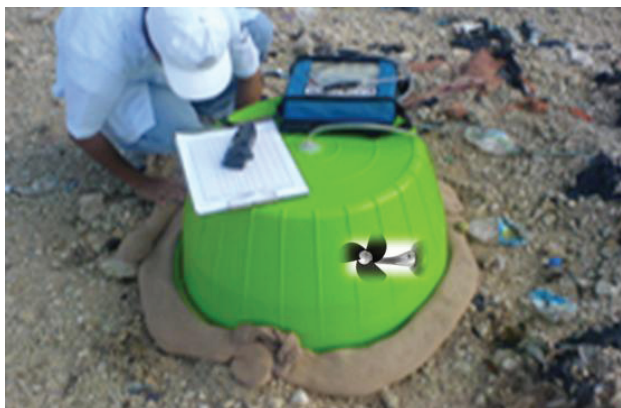
Figure 2. Static chamber technique applied in Merida landfill
