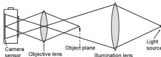
FIGURE 1. Generic diagram of a shadowgraph system.
