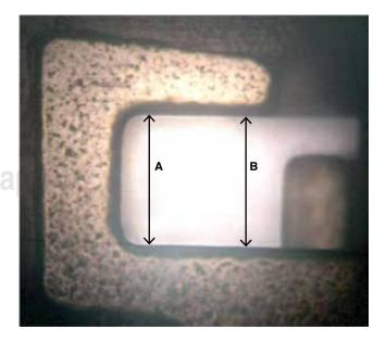
Figure 1. Internal (A) and external (B) measurements.
