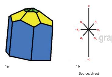
**Figure 1.** Schematic representation of hydroxyapatite cristal (a) and axes whereon those crystals are oriented (b).
