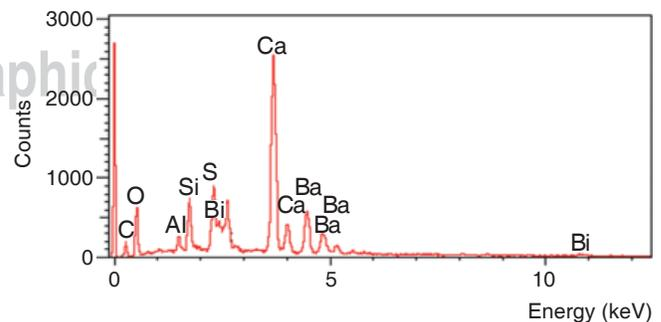
**Figure 6.** Chemical components detected in MTA CPM® are: Ca, Si, O, C, Mg, Al, S, Bi, and Ba.
