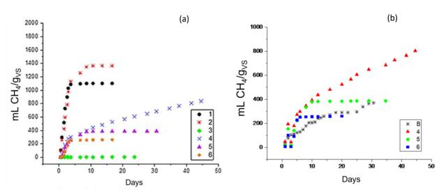
**Figure 6. (a)** Comparison of accumulated methane production under experimental conditions in Experiment II. **(b)** Comparison of accumulated production under experimental conditions with 50% vinasse and 50% elephant grass broth, from assays I and II, with and without addition of sodium bicarbonate. %V/C/A (alkalizer): 1 (50/0/50), 2 (75/0/25), 3 (0/50/50), 4 (50/50/0 - 0.05), 5 (50/50/0 - 0.11), 6 (50/50/0 - 0.25) e %V/C: B (50/50).
