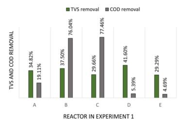
Figure 2. Variation of TVS and COD removal in the reactors of the Experiment 1.
