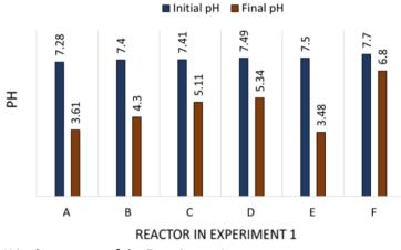
Figure 1. Variation of pH in the reactors of the Experiment 1.
